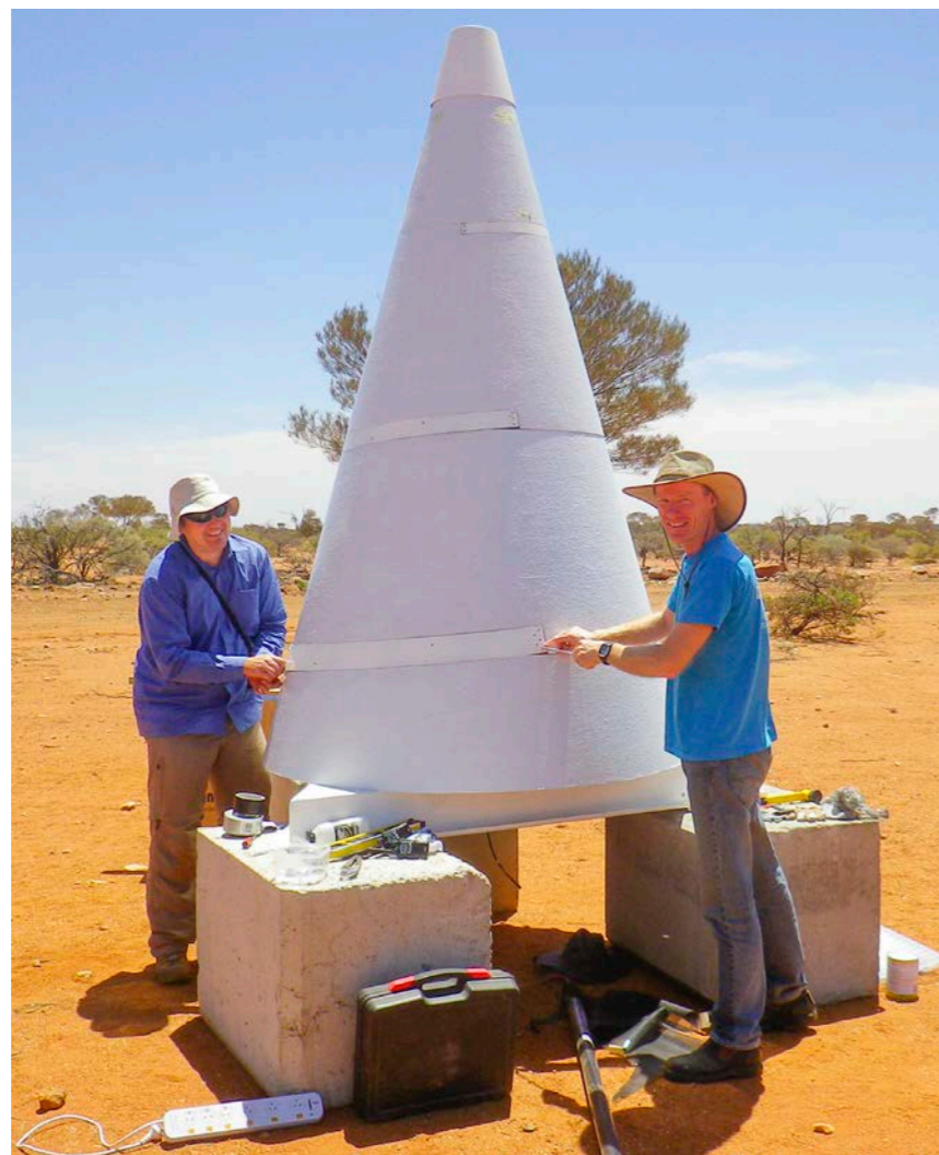
57. Dr Marcin Sokolowski and Dr Randall Wayth installing the BIGHORNS cone antenna at the Murchison Radio-astronomy Observatory.
